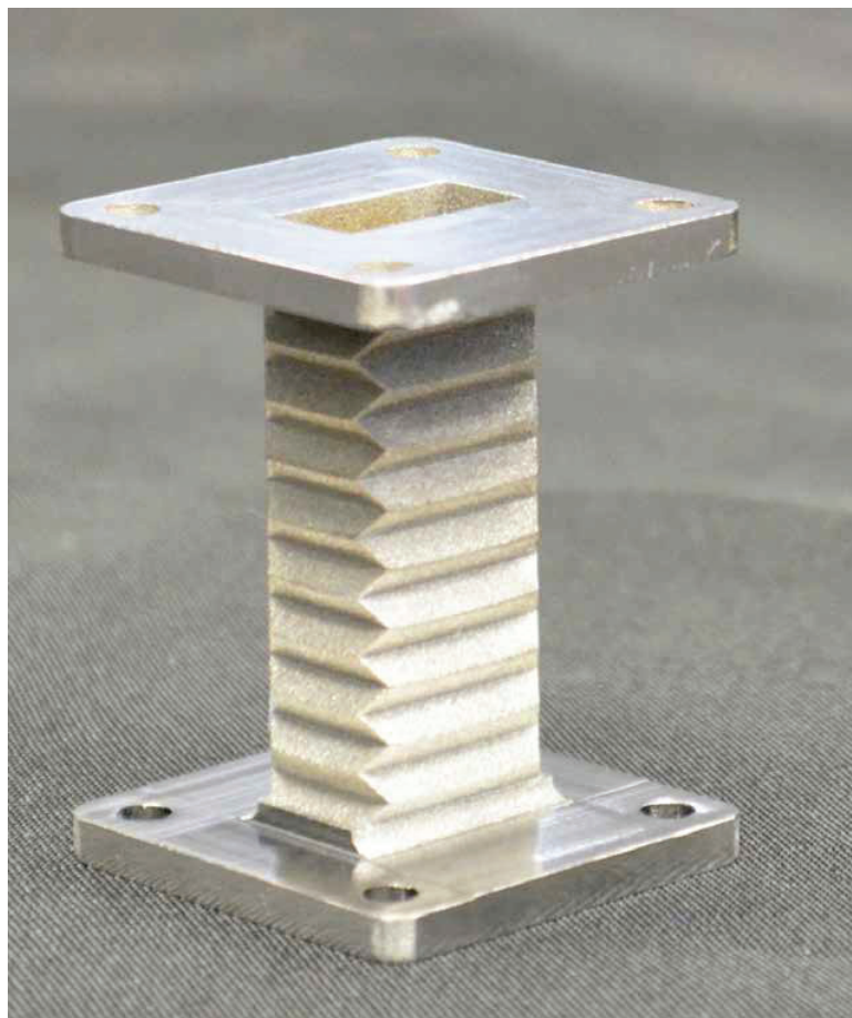
Fig. 13 Compliant AM shape-memory alloy NiTi microwave waveguide prototype. Rectangular cavity section dimensions: 8 x 16 x 38 mm (Courtesy of the authors/Penn State, supported by NASA SST programme)
