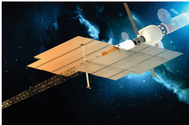
Fig. 1 Concept rendering of a proposed nuclear electric propulsion (NEP) spacecraft for Mars transit, designed to shorten Earth-Mars travel times. A 2,500 m 2 array of Modular Assembled Radiators for NEP Vehicles (MARVL) is shown to reject ~4 MW of heat (Courtesy NASA)
